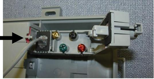
Figure 4: Plug telephone cord into the jack.
