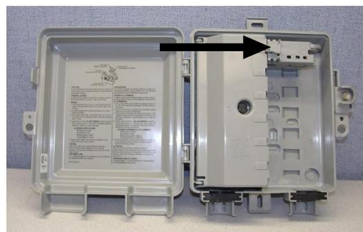
Figure 2: Release latch on modular jack.
